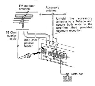
**CAUTION:** Never make a connection to a gas pipe because it can cause a fire hazard.
